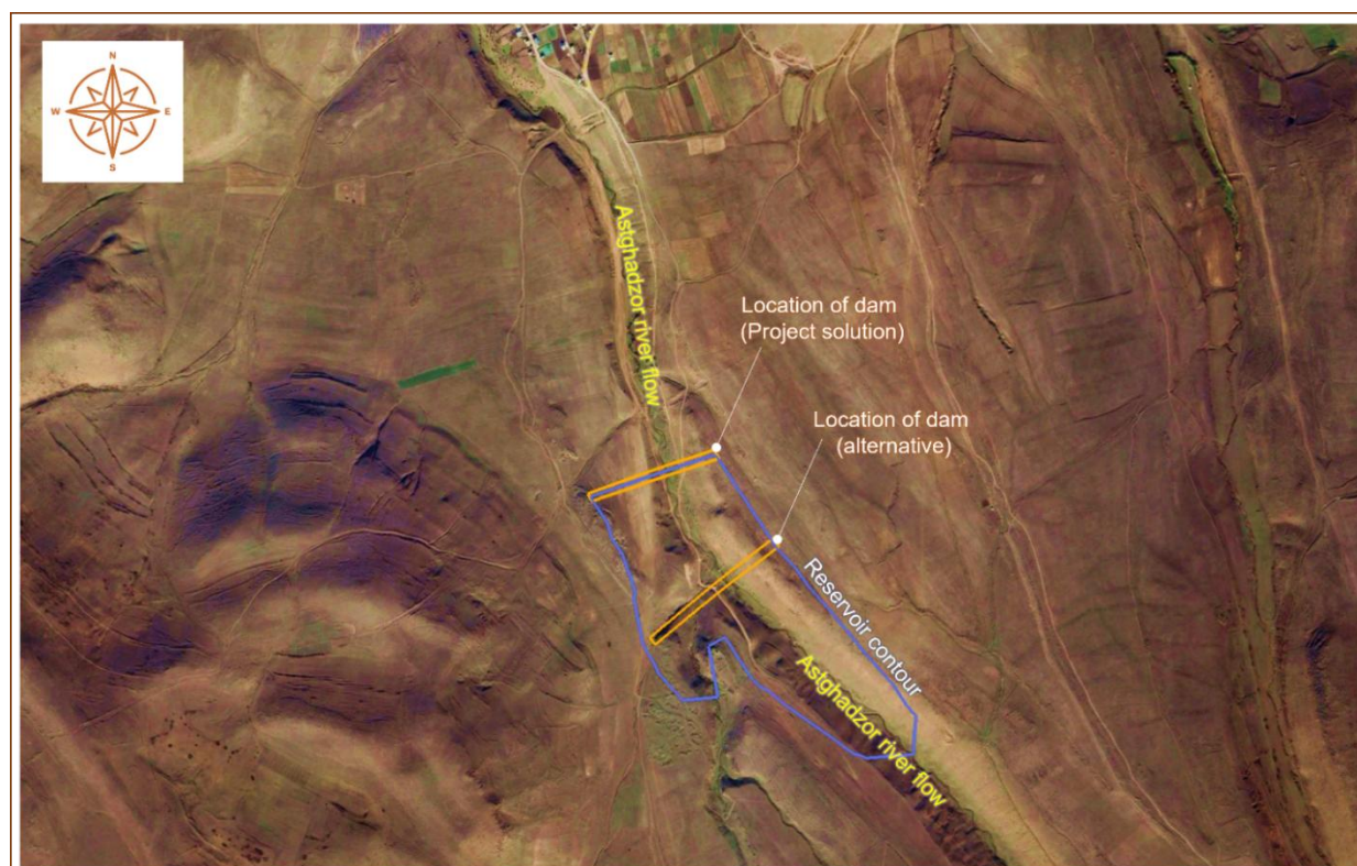
Figure 3-3. Alternative locations for the reservoir dam upstream the Astghadzor River
